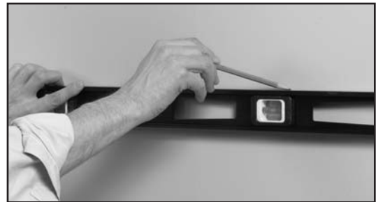
Fig. 17 – Use a level to establish vertical and horizontal lines.
