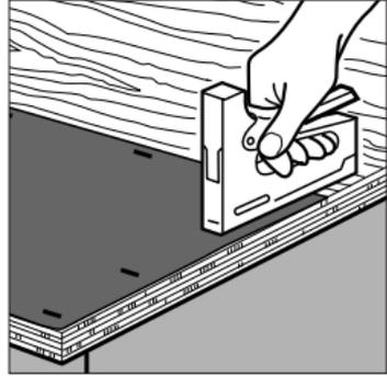
Fasten to the plywood with 1-1/4" DuRock Brand Wood Screws or 1-1/2" hot-dipped galvanized roofing nails, spaced 8" o.c. in both directions and around edges. Leave a 1/8" gap between panels.
