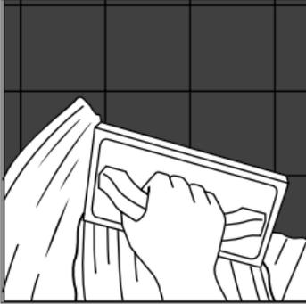
Fill joints completely. Remove excess grout with a float or squeegee as you go along.
