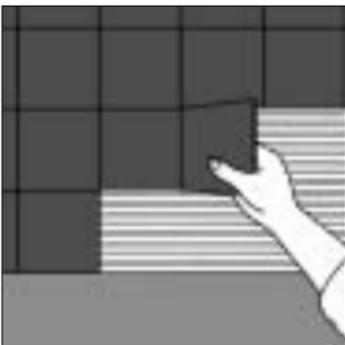
Maintain 1/4" shims beneath the bottom row of tiles and cement board to make a caulk joint along tub rim.
