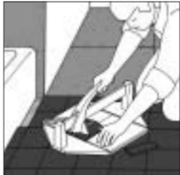
To make contoured and irregular cuts, use nippers to take small bites to prevent cracking or breaking of tile. With rod saw use long, even strokes to avoid binding. Smooth cut edges with an abrasive stone.
