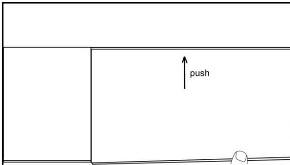
10. **Figure 4:** Using gentle force and at a 20-30 degree angle, push the long side tongue into the groove of the adjoining plank by sliding along the short side seam. You may need to lift the plank to the left of it slightly to allow for the “sliding” action.
