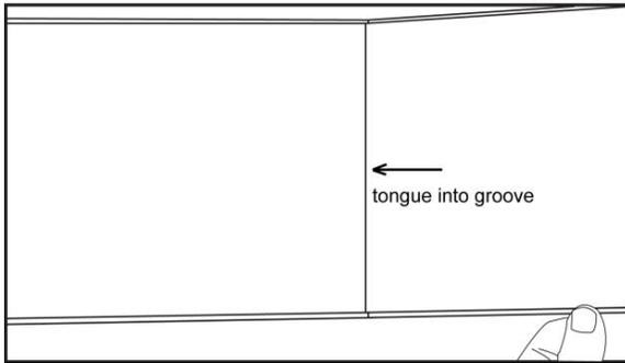
7. To start the second row, cut a plank that is at least 6" shorter than the first plank in the first row (you may use the left over from the last plank of the first row). Then install this first plank by inserting the long side tongue into the groove of the plank in the first row.
