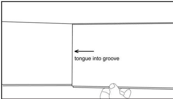
9. **Figure 3:** Align the plank so the long side tongue tip is positioned just over the groove lip of the plank in the first row.
